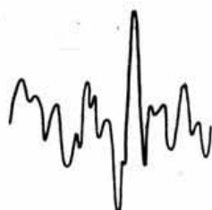
Fig. 1. Typical speech wave-form, showing relative infrequency and asymmetry of major peaks.
